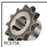
PCS75K Chain sprocket with hardened teeth, 19.05mm (DIN12B-1)
