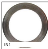
IN1 Internal gear, Steel 20NCD2
