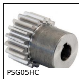
PSG05HC Skive hobbed spur gears - precision range, Case hardened steel 20NCD2
