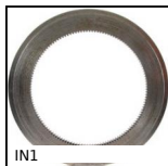
Internal gear, Steel 20NCD2
