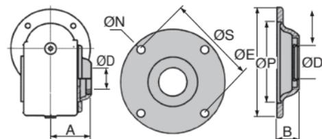
Open cover RFV-CAP-AT/SS and RFK-CAP-AT/SS
