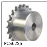
PCS625S Chain sprocket - Stainless steel, 15.875mm (DIN 08B-1)
