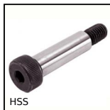
HSS Shoulder screw ISO7379, Hardened Steel class 12.9
