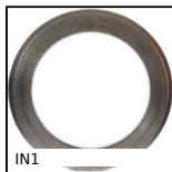
IN1 Internal gear, Steel 20NCD2
