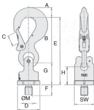
**4** Suitable for lifting in any direction
