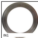
IN1 Internal gear, Steel 20NCD2
