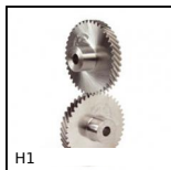
H1 Crossed helical gear crossed axis at 90°, Steel 20NCD2
