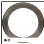
INO Internal gear, Steel 20NCD2
