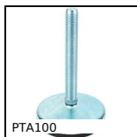
PTA100 Articulated levelling foot, pressed base Ø100, 15000N
