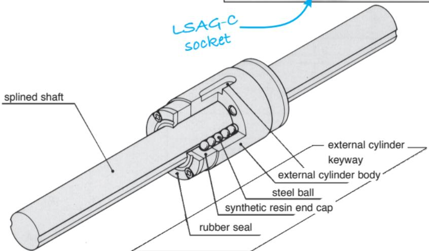
The LSAG series of linear ball splines consists of a splined shaft and an external cylinder. Two rows of rotating balls are housed in the external cylinder and turn on tracks in the shaft. These tracks have been precision-ground and allow **an almost unlimited lateral movement**. The splines stop the cylinder from rotating around the shaft. **It is therefore impossible to drive the cylinder in rotation.** The splined shaft and the external cylinder can be replaced easily.
