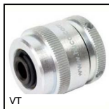
VT Vari-Tork® slip friction clutch, 0.53 to 1.32 Nm
