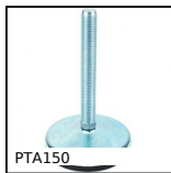
PTA150 Articulated levelling foot, pressed base Ø150, 40000N
