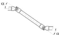
Entry and exit shafts should be parallel
