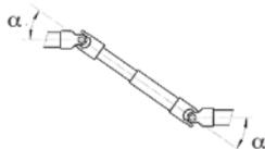
Shafts should be guided by bearings as close to joint as possible to reduce radial loads.
