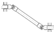
for constant velocity movement, the two angles should be equal and in the same plane
