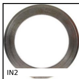
IN2 Internal gear, Steel 20NCD2
