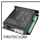
FIRSTDC1Q60 Speed controller 10A, 10 A
