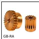
GB-RA Brass spur gear, Brass CuZn39Pb3
