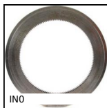
Internal gear, Steel 20NCD2
