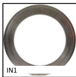
IN1 Internal gear, Steel 20NCD2
