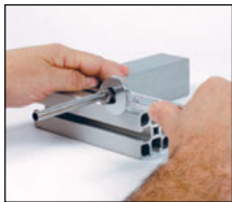
Position and then lock into place using a spanner
