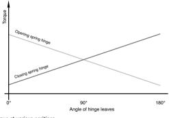
M: hinge torque at various positions  $M(o^\circ)$ : torque when hinge leaves are parallel  $M(90^\circ)$ : torque when leaves are at 90°  $M(180^\circ)$ : torque when leaves are at 180°
