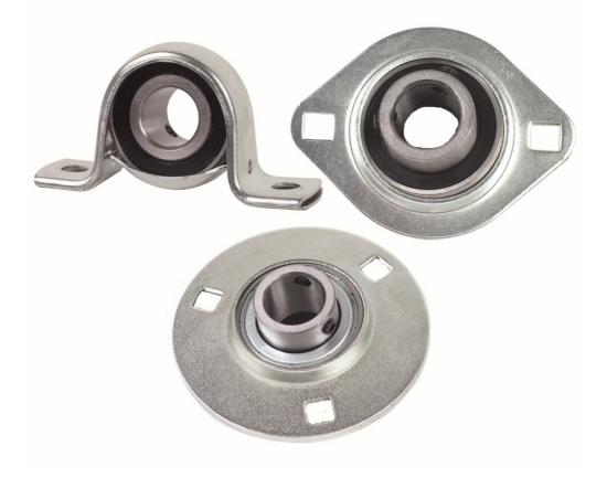
This new range of sheet metal bearings marketed by ENGRENAGES HPC are complete, ready-toinstall units consisting of self-aligning bearings in either surface-mounted or cap-type housings. These bearings compensate for misalignment of the shaft and are self-aligning as they have ball bearings that are in radial contact with large inner rings and sealing gaskets. The flanged housings have 2 or 3 mounting holes, the cap bearings have a base plate with 2 mounting holes.
